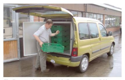
The Euro-transCooler 8 for eight Euro crates is available as a standard refrigerating unit with a temperature range of  $+2^{\circ}$  to  $+10^{\circ}$ C. The Euro-transCooler 8 TK offers you an extended temperature range from  $+15^{\circ}$  to  $-25^{\circ}$ C, so that you can also use it to transport frozen products.
