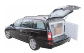
The Alpha GTA Dig, which was specially designed for use in station wagons, is particularly powerful and can be used for transporting both refrigerated and frozen products.
